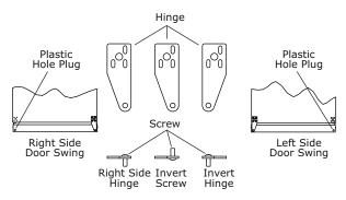
10. Remove pivot screw from top hinge, invert screw and reinstall pivot screw in top hinge.
