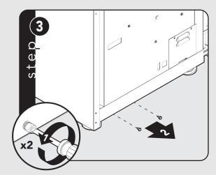
Remove two screws from back of range.
