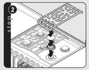
Burner heads and burner caps are packed in the cardboard top pack with the grates. Align burner head on burner base. Place burner cap on burner head. Place grate onto the burner pan.
