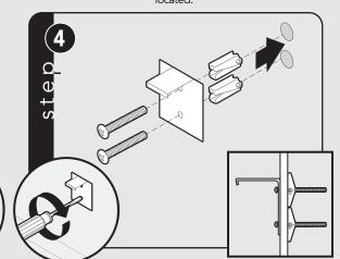
Attach bracket with mounting hardware provided.
