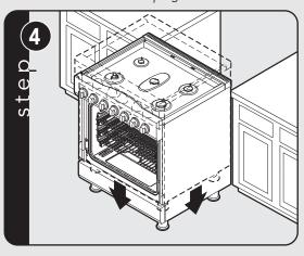
Lower range gently to keep any undue strain from legs and internal mounting hardware.
