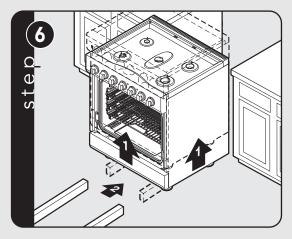
Lift unit and prop on wood blocks.
