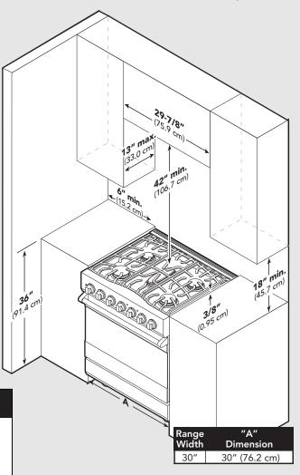
**Note:** If a range hood is installed, wall cabinets above the range have a different minimum clearance height.
