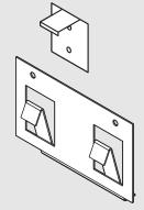
**Important:** The range **MUST** be installed with one of the anti-tip devices.
