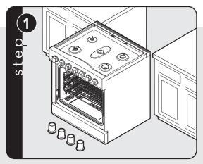
Legs are packed in the cardboard top pack. Note: Legs should be installed near to where appliance is to be used, as they are not secure for long transit.
