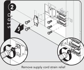
bracket and three supply cord mounting screws on terminal block.
