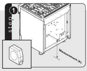
Measure from floor to bottom of the anit-tip opening located on the back of range. This will be measurement (A).
