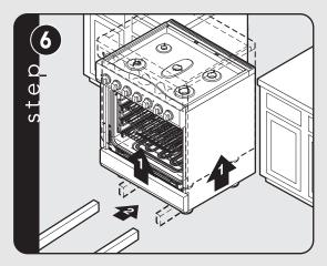
Lift unit and prop on wood blocks.
