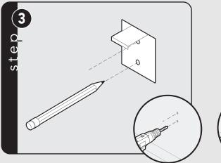
Mark and drill holes where bracket will be located.
