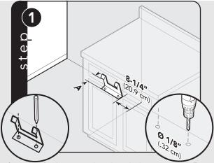
Refer to chart for dimension A based on whether or not standoffs are used with the rear trim device. Mark and drill 1/8" (.32 cm) holes where bracket will be located
