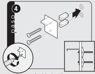
Attach bracket with mounting hardware provided.
