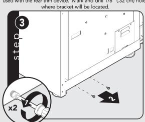
Remove two screws from back of range.
