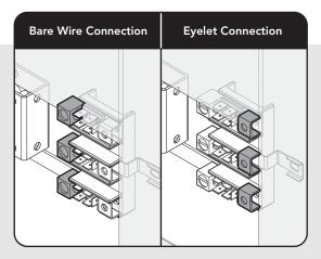
To make a bare wire connection, use holes on the left side of the terminal block. To connect eyelet style wires, use holes on right side of terminal.
