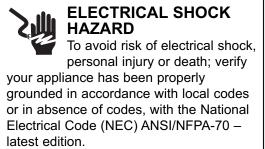
Use a 3-wire power supply cord kit rated for 40 amps – 125/250 volts with closed loop terminals and marked for use with ranges.
