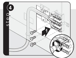
Attach line #1 (black) and line #2 (red) leads to outside terminal. Attach neutral wire (white) to center terminal on the terminal block.
