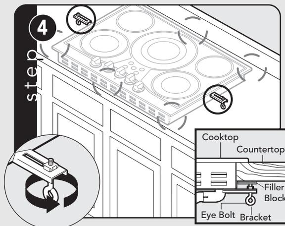
Screw sheet metal screws into brackets and tighten firmly against bottom of countertop.
