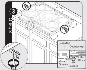
Screw hold down brackets to the burner box using the #10 x 1/2" sheet metal screws. There are 6 bracket assemblies included. There must be a minimum of 2 brackets installed with the possibility of up to 6 in locations noted depending on installation
