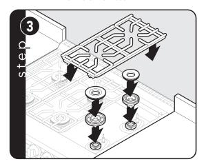
Burner heads and burner bases are packed in cardboard top pack with the grates. Place the burner base on top of the burner flange and the burner head on top of the burner base. Place burner grate on top of grate support.
