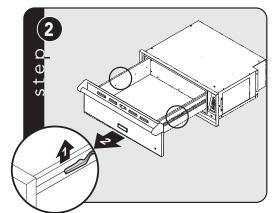
Slide finger along right and left side until you reach the hand latches (located approximately in the center of the rail). Pull up on on the left side latch and press down on the right latch at the same time and pull out the drawer pan.
