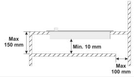
IMPORTANT: In case of installation on an empty kitchen unit with doors, a separation panel must be placed under the hob, which must be easily extractable to allow sufficient access for any technical assistance.
